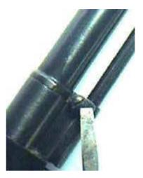
ejector rod spring retaining screw - after takedown
