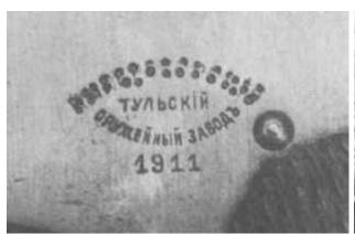
First line of the marking, punched out
