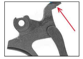
The picture below shows the position of the parts after the hammer was thumb-cocked, and caught by the sear (red arrow here-left), which is an integral part of the rear arm of the trigger.
