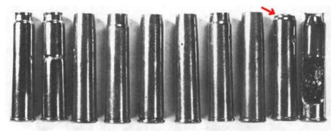
series of 7,62 mm ammo - The red arrow points onto a Fiocchi with a shorter case.
