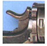
In 1883, a new cheaper Nagant model was used by the Belgian Army. The cylinder periphery was plain, without the usual lengthwise flutes, and the lock was of single-action type as shown in the two pictures here (the hammer must be thumb-cocked for each shot). Also, the hammer was of rebounding type. In the picture on the left, the hammer is positioned slightly rearward when the trigger is released.
