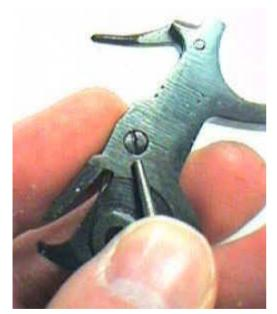
double-action hammer with a strut
