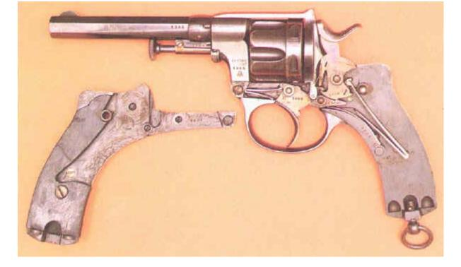
Internal mechanism of the Nagant Model 1878 - © B&B
