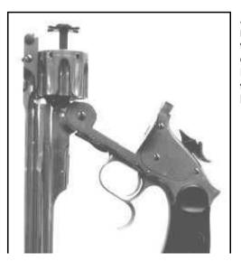
Anotherdrawback of the Nagant was the obsolete loading system that was retained. Even if the loading gate principle was in very wide use at that time, the trend was to equip up-to-date revolvers with a side-swinging cylinder combined with an effective collective extractor like the one used in the French model 1892 (picture below), or at least to use a top-break system, like those that fit the old Russian Smith & Wesson service revolver (picture hereleft) or some of the English Webley revolvers.
