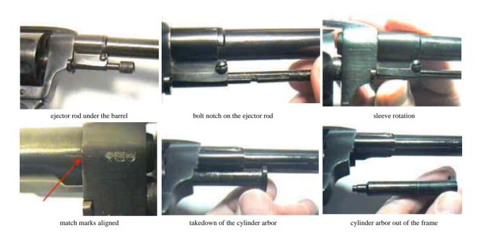
Once the cylinder arbor is removed, open the loading gate on the right side and take out the cylinder toward the right. The cylinder bears a bushing that can be extracted by first turning it until its small lug aligns with an exit track in the cylinder. The bushing then pops up under the pressure of its spring.
