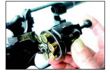
In the Nagant case, every spent cartridge had to be pushed out individually by the ejector rod that pivoted around the barrel. Moreover the rod was even not equipped with a return spring. This obsolete feature for a service revolver made the loading and unloading operation both lengthy and very tedious. Many Russian officers were very happy to keep their old easy-to-load and powerful Smith & Wesson revolvers when fighting against Japan (1904-1905) and even as late as WW I against Germany.
